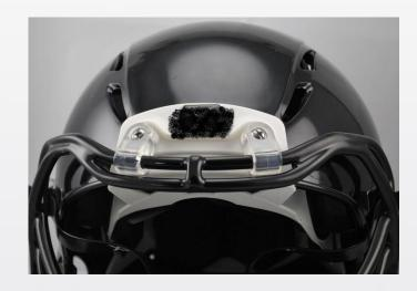
Some loop straps are NOT accessible to a standard cutting tool (eg FM extractor) in its placement as it relates to the facemask in order to remove the entire facemask.
